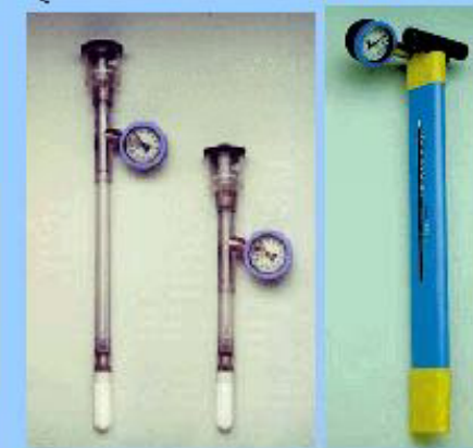
Soilmoisture's JetFill & Quickdraw Portable Tensiometers
